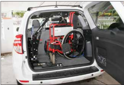
The wheelchair hoist makes it easier to lift and store Cathy Palanganas' wheelchair in the back of the family vehicle. The hoist was purchased through the assistance of a GOAL-AT Loan, administered by the GSAT Center.
